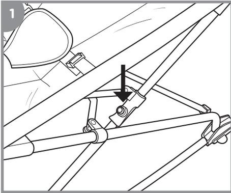
Press Lock Buttons on each side until you feel the Buttons release.
