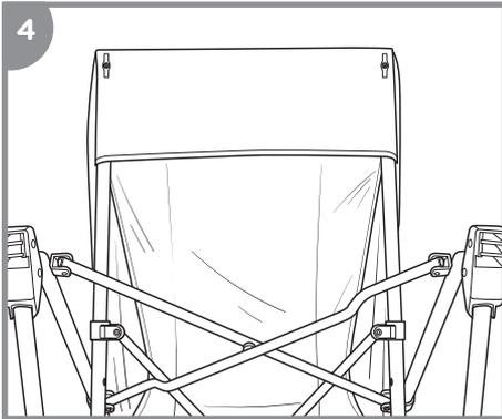
To assemble the Cover, secure Cover with Cleats fed through the two slots in upper back area of cover.
