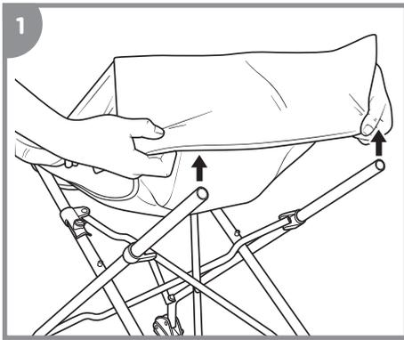
Pull Cover off the two Cleats and remove Cover from Frame.
