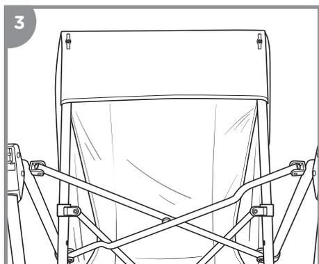
3 To re-assemble the Cover, secure Cover with Cleats fed through the two slots.
