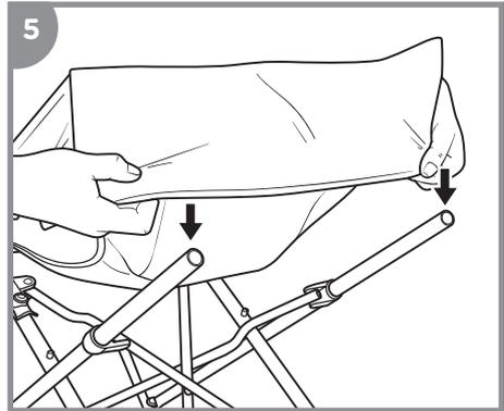
Pull bottom of Cover over bottom of Frame.
