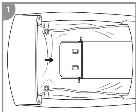
1 Insert large Plastic Support back into Pocket and thread two Harness Buckles through slots.
