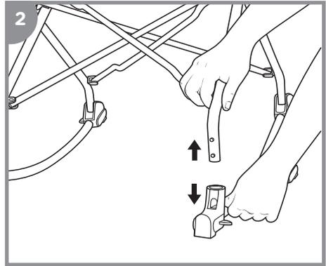
Press Buttons on Front Legs and lift Legs out of Front Feet.
