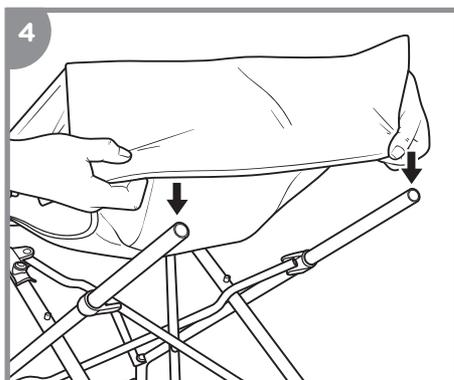
4 Pull bottom of Cover over bottom of Frame. Refer to "Assembling the Rocker" section to complete assembly.
